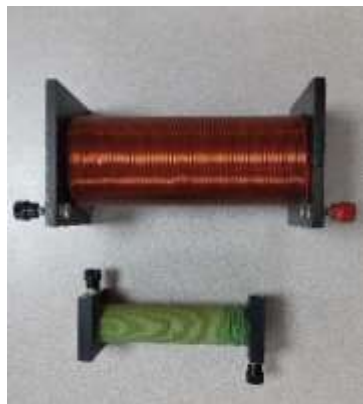
Figure 1: The big solenoid is the primary solenoid, the small one the secondary solenoid.
