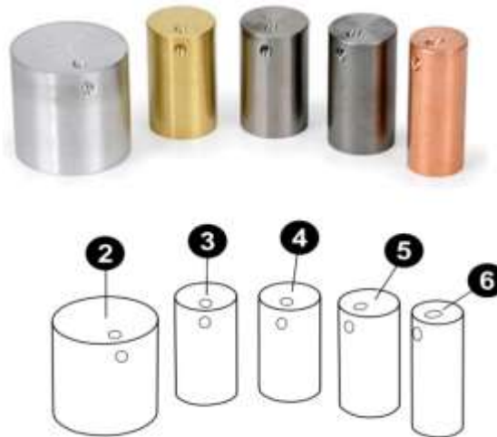
Figure 1: (2) Stainless Steel. (3) Brass. (4) Aluminum. (5) Zinc. (6) Copper
